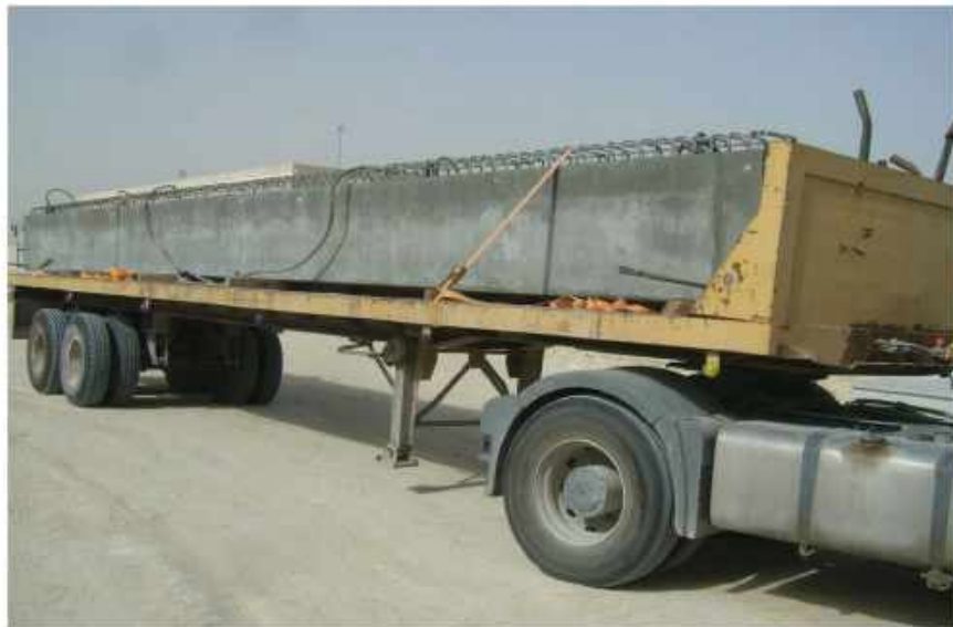
Precast Bridge Girder for SRO
